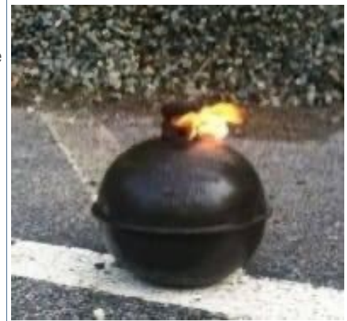
Smudge pot used in road construction up until the 70's to warn motorists of repair work ahead. Before blinking lights construction workers and the rail road used these pots to alert motorists to be extra cautious in work areas.
